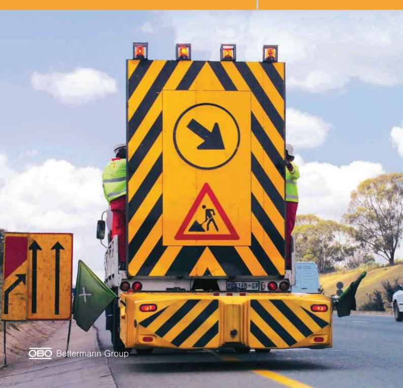
The Alpha 70K Truck Mounted Attenuator meets NCHRP 350, Test Level 2 criteria and offers a wide range of protection for workers, motorists and equipment.
